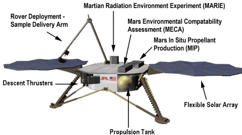
**Fig. 1:** The 2001 Mars Surveyor Lander, showing the five experimental payloads (MECA, MARIE, MIP, MARDI, and APEX).
