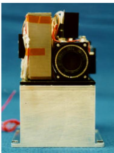
**Fig. 3:** A view of a chemistry cell and actuator assembly.
